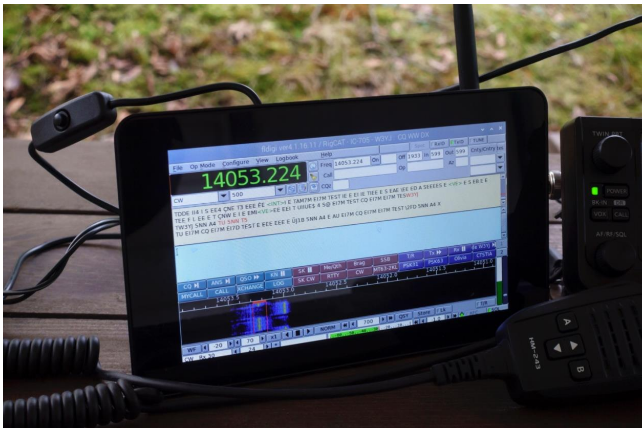
Fldigi running on a 7 inch touch screen tablet based upon a Raspberry Pi 3B+
