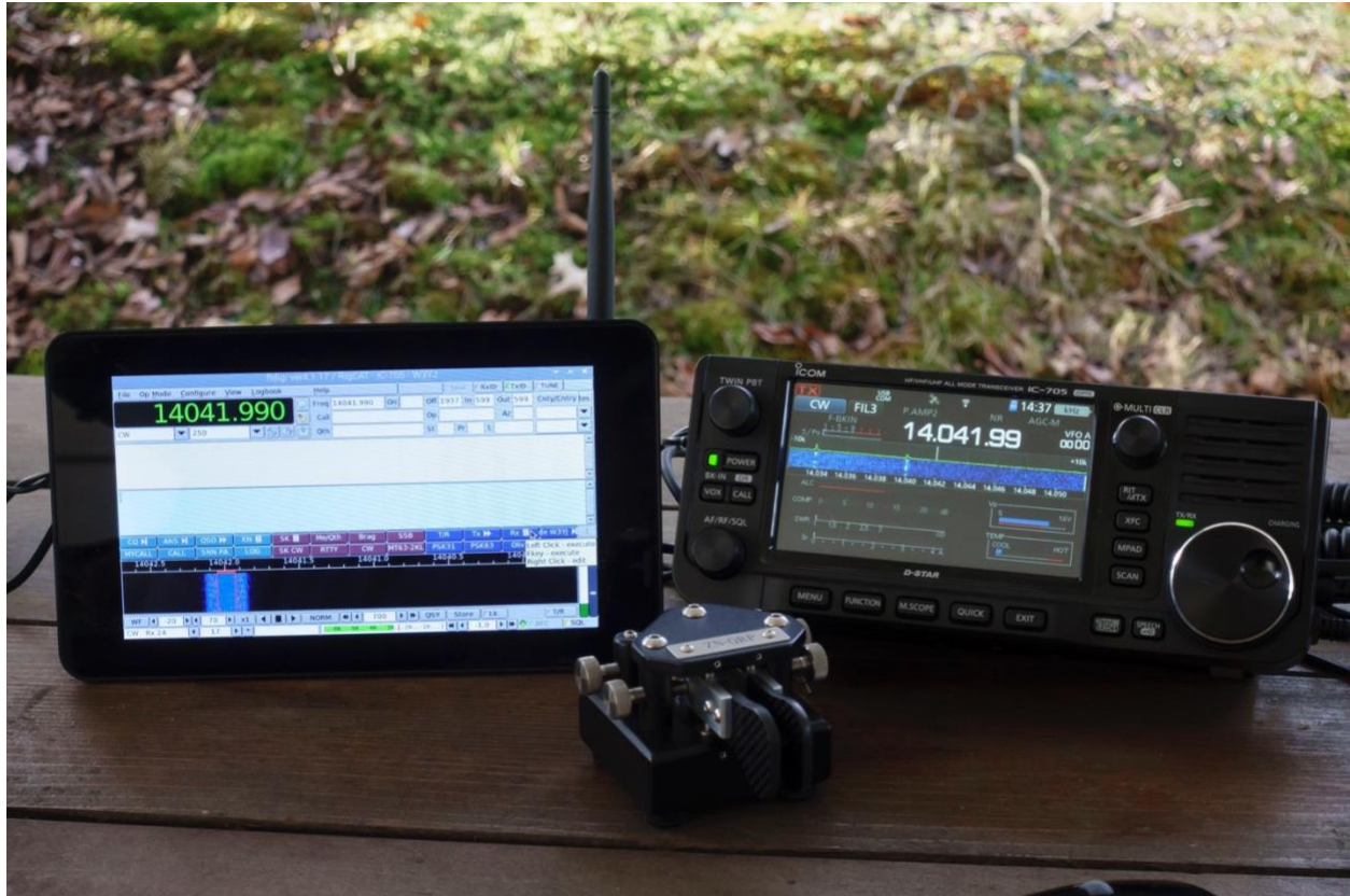
Raspberry Pi 3B+ tablet with Icom IC-705 and N3ZN ZN-QRP CW paddle. The “rubber duck” antenna on the tablet is for wi-fi, the built-in wi-fi antenna on the Raspberry Pi 3 is very poor.
