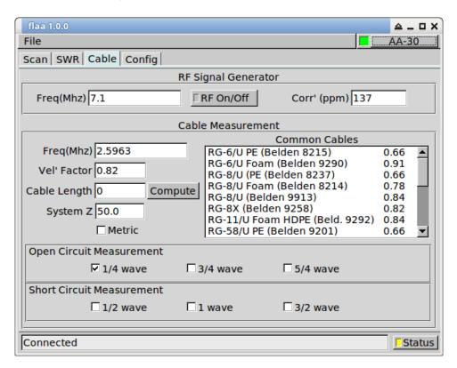
Either enter the cable velocity factor, or select from one of the common cables control. The input impedance to an open circuit coaxial cable will be 0 + j0 at 1/4, 3/4, 5/4 ... wavelengths. An open circuit cable will be at 1/2, 1, 3/2 ... wavelength.
