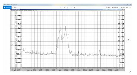
One of the popular EMCOMM modes a few years ago was the very robust **OLIVIA 8-500**. Olivia can decode to very low signal/noise ratios (below -10 dB) but Olivia has long delay times from when tones are heard to when print appears on your screen. Long delay times drag out the time for check-ins on a busy net. **Olivia 8 – 500** has 8 tones, sent one at a time, 63 baud, 500 Hz bandwidth and an overall speed of 30 wpm. It might be the mode of choice for very faint signals under poor propagation.
