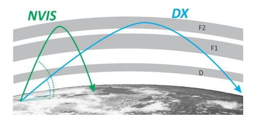
Typical NVIS paths get into the deep valleys. Transmitting antennas need not be on the hilltops
