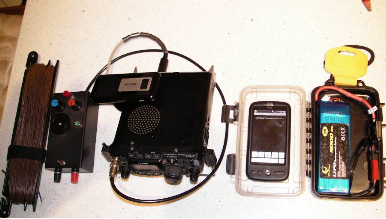
The whole portable set-up: 41M wire and tuner for end-fed Fuchs antenna, FT-817 with Bluetooth adapter, Android phone, 5Ah battery in sealed box.
