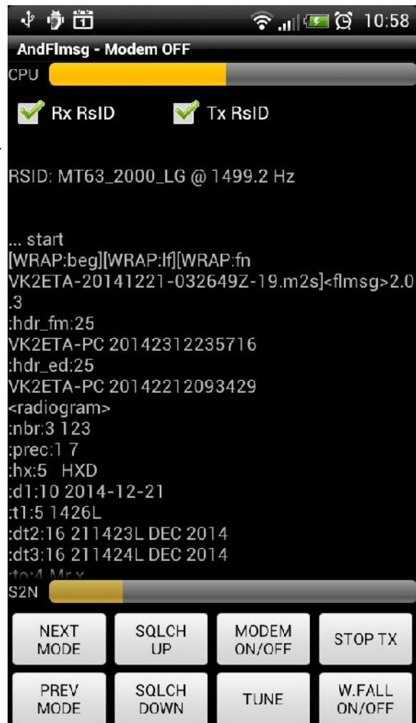
**Be aware that the CPU load increases when displaying the waterfall and on some (old and slow) devices doing so while on multi-carrier PSKR or any of the THOR modes can lead to losses of data AND making RSID not detectable.**
